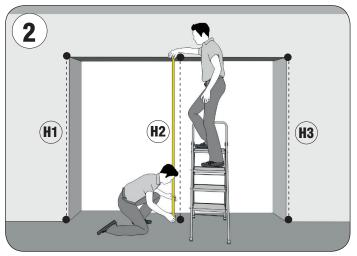
Measure the opening height (H) from clean floor. For proper measurement make sure that measurment tame on same possition. Record the maximum value.  $\mathbf{H} =$
