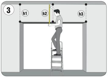
Measure the headroom of the opening (h). If beams, cables, ventilation ducts pass in the area of the headroom please write a note on the first page.
