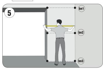
Measure the left wall (br) to the nearest obstacle (pipe, box, wall, etc.). Write down the minimum value.
