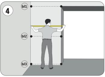
Measure the left wall (bl) to the nearest obstacle (pipe, box, wall, etc.). Write down the minimum value.
